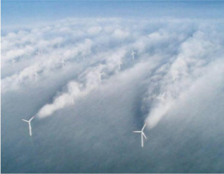
Figure 2.11: Visualization of wakes in an offshore wind farm [26]
