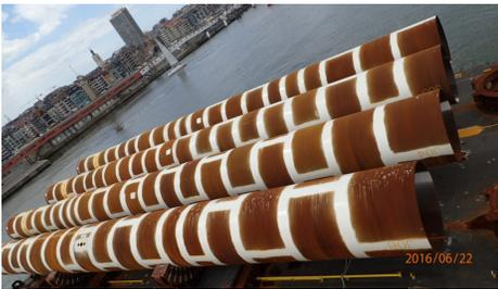
Figure 1.8: Different elements are welded (white areas) together to form the monopile foundation of an offshore wind turbine. [11]
