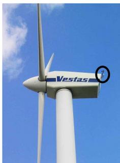
Figure 1.10: The anemometer (encircled in the figure) used to measure wind speed and wind direction is usually located behind the rotor of the turbine [16]
