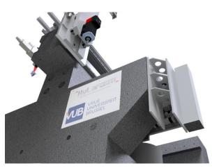
behaviour of this in-house developed machining platform. The interaction of the machine frame stiffness and mass on the one hand, and the motion components such as bearings and linear motors on the other hand are to be quantified or simulated.
